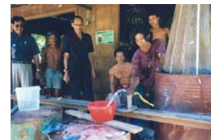
Miner in Guha, Kahayan River using the RHYP retort (burning with gasoline torch)
