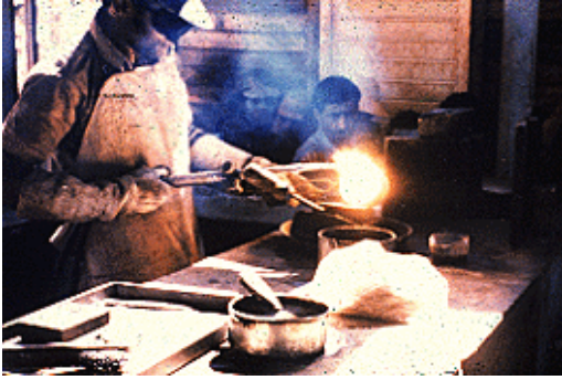
Retorted Au (still with Hg) is sold to gold shops and melted: Hg vapor is released in the villages...
